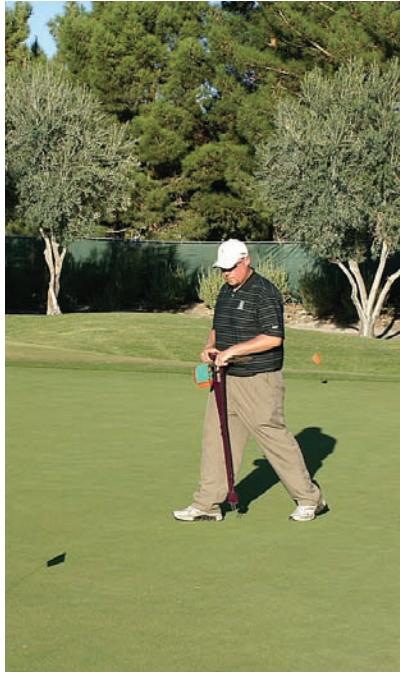
TPC Summerlin's Dale Hahn, CGCS, champions the TDR 300 soil moisture sensing device in his water management program. Pictured is Dustin Peterson, assistant superintendent at TPC Deere Run in Silvis, Ill., taking a reading at TPC Summerlin during a 2011 PGA Tour event. Photo by Dale Hahn
